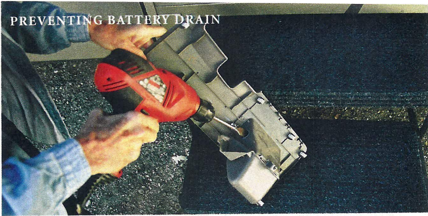
Check clearance and drill a 3/4-inch hole in the lower dash panel coin pocket.
