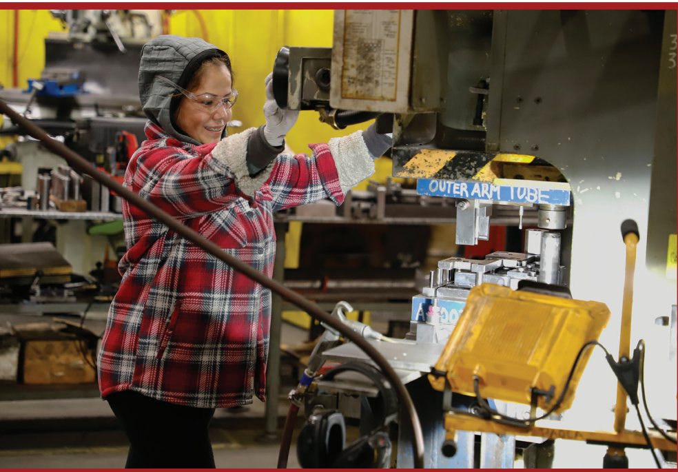
Paula Rojas operates a punch press to stamp out parts and subcomponents.
