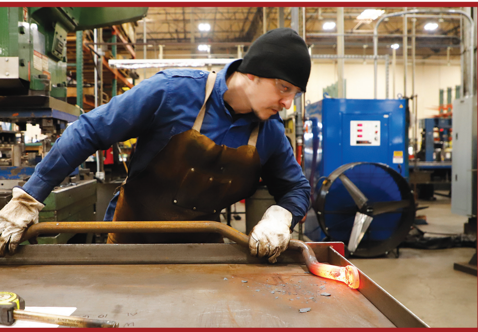
Andrey Zagorulko verifies the mounting tab alignment on a newly forged sway bar. Tow bars are allowed to cool after the metal is forged.
