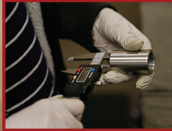
Roadmaster continually checks parts specifications for proper tolerance even during the manufacturing process.
