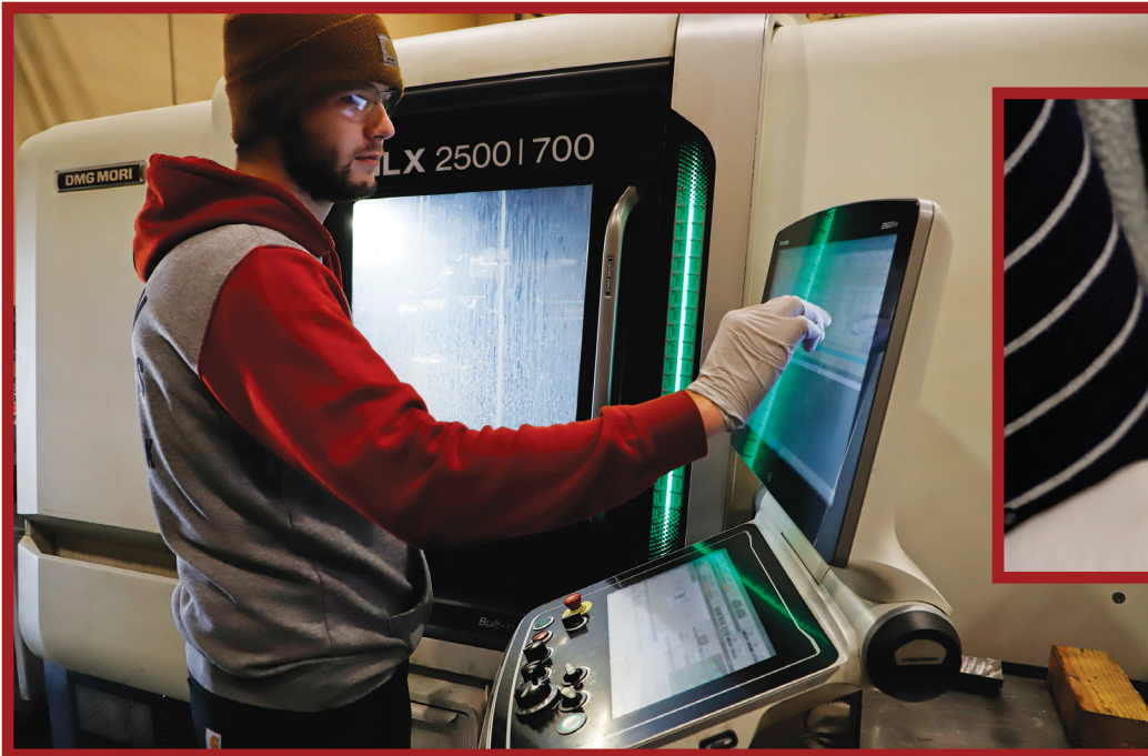
Andrew Kolberg sets up a CNC turning center for parts production.
