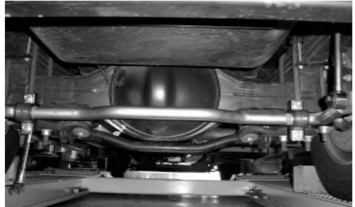
\*Before you begin, inspect the vehicle's U-bolts that will be reused in the installation of this kit. Consider replacing them if they are rusty or show other signs of structural wear.\*
