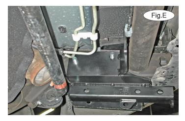
3. Set the main receiver brace in place against the inside edge of the frame rail and over the 5/8" x 5" bolts (Fig.E). Bolt into place using the supplied 5/8" lock washers and nuts (Fig.F). *Note:* the power steering cooler line may need to be bent slightly to allow for clearance of the main receiver brace.
