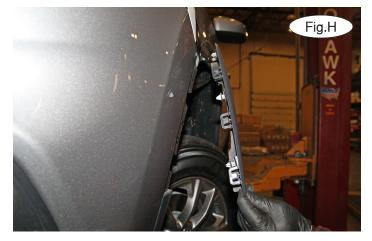
4. On each side, remove four 8mm (head) screws attaching the fender liner to the fascia (Fig.G). Pull back the fender liner and remove one 10mm (head) bolt (Fig.G – inset). On each side, pull out on the corner of the fascia to release the locking strip and the wheel well trim clips (Fig.H). Then, use a panel tool or similar to carefully pull down on a plastic retaining clip (Fig.I) and at the same time, pull out on the corner of the fascia to release it (Fig.J).
