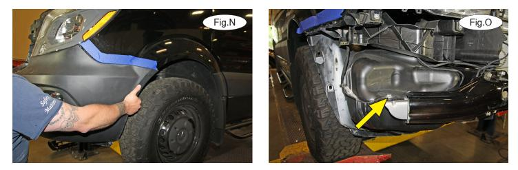
8. For models without a Diesel Emission Fluid tank: Skip to the next step. For models with the tank: On the passenger side only, remove one 13mm (head) bolt attaching the reservoir to the bumper core (Fig.O).
