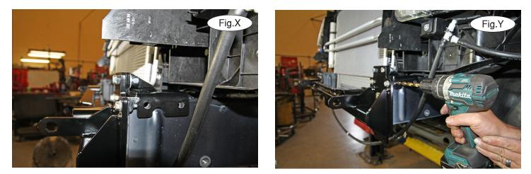
15. Working on the driver's side only, place the upper rear brace over the frame rail, aligning its holes with the top mounts on the main receiver brace. Loosely bolt the upper rear brace to the main receiver brace using the two supplied  $3/8" \times 114"$  bolts, and then finish with small 3/8" flat washers, 3/8" lock washers and 3/8" nuts (Fig.X).
