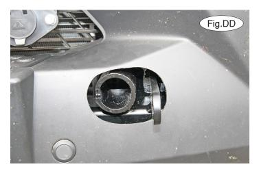
20. On each side, trim the fascia as needed to allow clearance for the arm and tab (Fig.DD).
