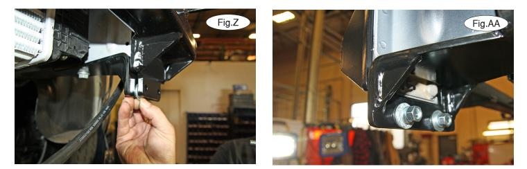
16. Use a 3/8" bit to drill straight through the side mounts of the upper rear brace and the frame rail. Bolt through the upper rear brace and frame rail using the supplied 3/8" x  $4\frac{1}{2}$ " bolts, and finish with 3/8" lock washers and nuts (Fig.Y). Then, tighten all bolts to the bolt torque requirements found at the end of these instructions. *Note:* use Loctite® Red on all nuts and bolts.
