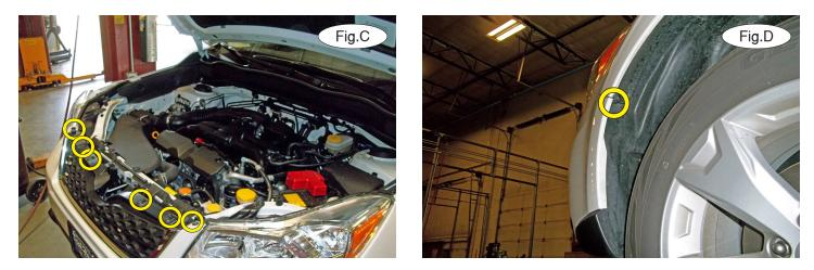
1. *Important:* please use all supplied bolts and parts and read all instructions carefully before beginning this installation. The majority of questions you may have can be answered within the text, and proper installation will ensure safe and secure travel. Now, begin the installation by removing six plastic fasteners attaching the fascia to the core support (Fig.C).
