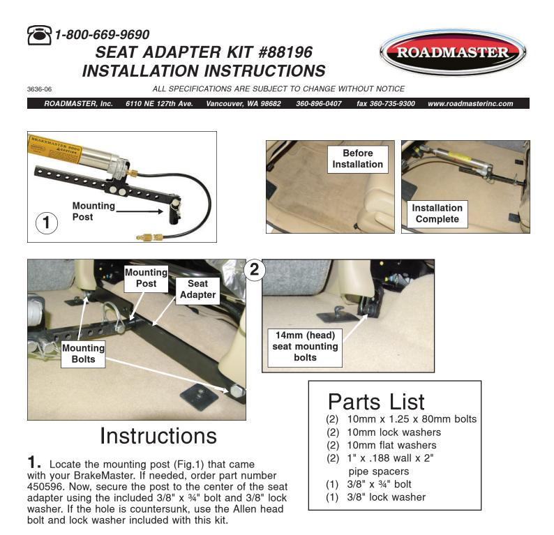
**2.** Start by removing the two 14mm (head) seat mounting bolts, located behind the plastic covers. Now, place the 1" x .188 wall x 2" spacers over the holes you removed the 14mm (head) bolts from. Set the seat adapter over the spacers and bolt into place using the supplied 10mm x 1.25 x 80mm bolts, flat washers and lock washers.
