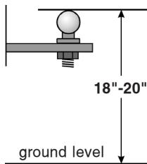
The coupler requires a two-inch hitch ball with a 5,000 pound capacity.
