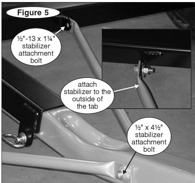
after the dolly is completely assembled.
