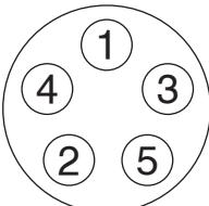
Use this crossing pattern to tighten the lug nuts.
