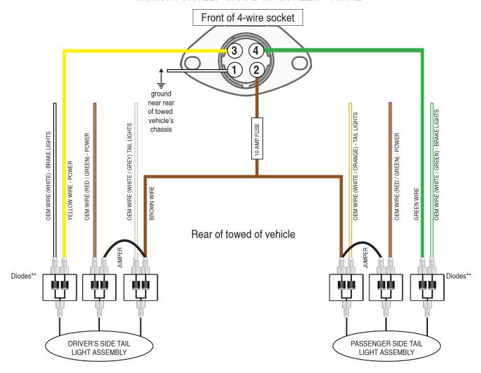
To power up the tail light assemblies on the Jeep Grand Wagoneer, simply plug in the dinghy to the motorhome and turn ON the headlights on the motorhome.
