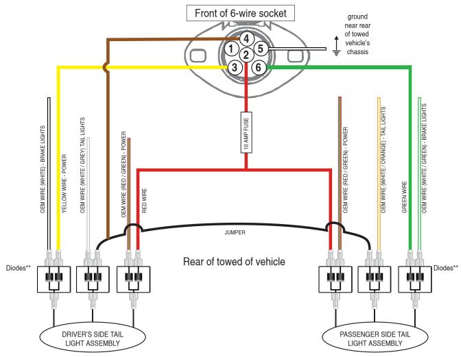
To power up the tail light assemblies on the Jeep Grand Wagoneer, simply plug in the dinghy to the motorhome. The 12V charging circuit will always have power.
