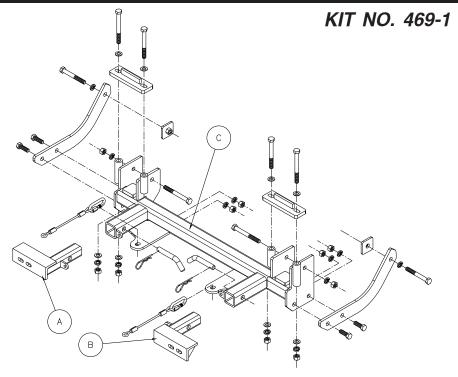
**IMPORTANT:** All baseplates **must** be assembled with all the bolts left loose for final adjustment and positioning (before tightening) unless otherwise instructed. All bolts **must** be torqued for proper strength. If more than one bolt is used per fastening point, the diagram may only show one. Use flat washers over all slotted holes and lock washers on all fasteners.
