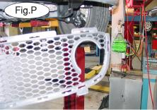
17. Reinstall grille and fascia by reversing steps 1 through 4. The standard grille will fit over the receiver braces without trimming (Fig.O). The turbo/s model grille will require trimming to fit (Fig.P).
