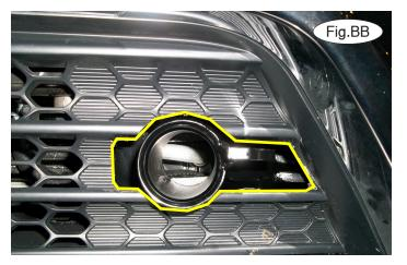
22. **If your fascia appears as in Figure AA or BB:** trim using the yellow lines as a reference. **If your fascia appears as in Figure CC:** Trim the front of the fascia (Fig.CC) and then the backside (Fig.DD) to allow clearance for the main receiver brace.
