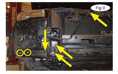
over a ½" x 2½" bolt and bolt up through the baseplate, pipe spacer and bumper core, finishing with a ½" flat washer, lock washer and nut (Fig.U). *Note:* If you are having fit issues with the pipe spacers, you may need to adjust the bumper. To do so, loosen the three 13mm bolts (Fig.V – yellow arrows) and permanently remove the 10mm bolt (red arrow). If the vehicle has air suspension, you may also need to loosen the two 13mm nuts Figure V (circles). *pg* 6
