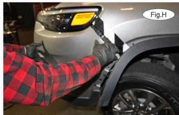
5. On the driver's side only, disconnect the electrical connector (Fig.I) and then remove the fascia and set it aside. *Note:* Make certain that the vehicle is not turned on while the connector is unplugged or it may trigger the 'Check Engine' light to illuminate.
