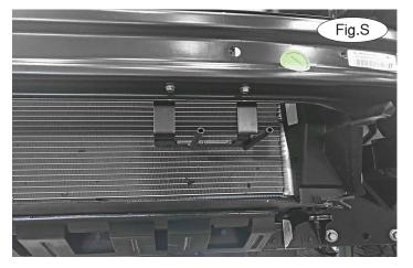
15. If you will be using the wiring plug plate that we provide, measure over  $8\frac{3}{4}$ " from the edge of the driver's side tow hook mount and drill a  $\frac{1}{4}$ " hole (Fig.R). Then, measure over another  $\frac{3}{2}$ " and drill a second hole. Mount the wiring plug plate to the bottom of the bumper core using the supplied two  $\frac{1}{4}$ -20 x 1" bolts and whiz nuts (Fig.S).
