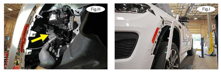
5. On each side, peel back the fender liner and unplug any wiring harnesses in the indicated area (Fig.H). *Note:* If the vehicle has a front camera washer, you will need to cap and secure that line as well.
