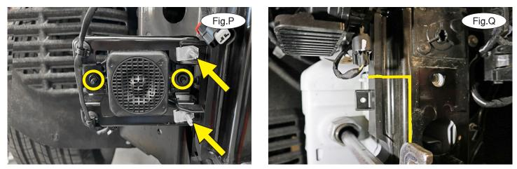
11. **If your vehicle does not have a pedestrian alert device (PAD):** Proceed to the next step. **If your vehicle has a PAD:** Remove two T35 screws attaching the PAD to its mount (Fig.P – circles). Disconnect the plug and its harness and remove two 10mm bolts attaching the factory PAD mount to the core support (Fig.P – arrows). It will not be replaced.
