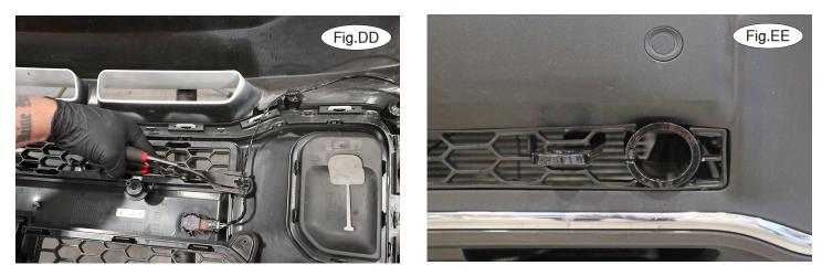
23. On each side, disconnect one wiring harness mount from the lower air dam opening (Fig.DD).
