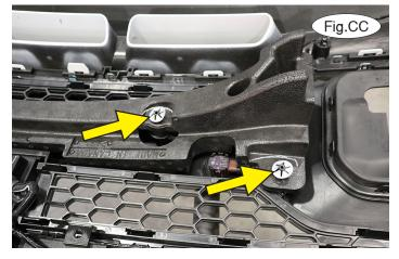
22. On each side, remove two star clips attaching the shock absorption pad to the back of the fascia (Fig.CC). Pull out to remove the pad. It will not be replaced.
