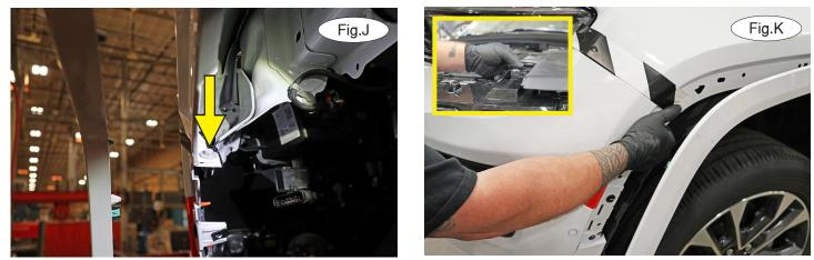
7. With the assistance of a second person, simultaneously pull out on the seam (Fig.K) and pull up on the top of the fascia to clear the hood bump stop (Fig.K – inset). Remove the fascia and set it aside for now.
