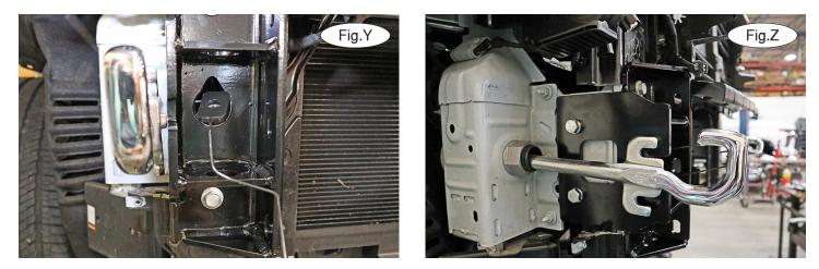
18. Place a  $\frac{1}{2}$ " lock washer and Loctite over two  $\frac{1}{2}$ " x  $1\frac{1}{2}$ " bolts. Locate the 3/16" x 1" x 2" threaded backing plates with rods. Bend the rods so the backing plates can be inserted into the frame and over the side mounts (Fig.Y). Then, bolt through the access hole you cut in step 16 and bolt into the backing plate for each hole (Fig.Z). Now, tighten the bolts to the torque specifications.
