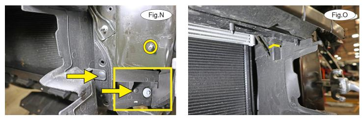
10. On each side, trim off the bumper core mounting stud (Fig.N – circle) using a cut-off wheel or a die grinder. Then, remove two Christmas tree fasteners attaching the lower air dam to the bumper core mounts (Fig.N and Fig.N – inset, arrows). Then, cut the air dam at the spot indicated (Fig.O) and remove it. It will not be replaced.
