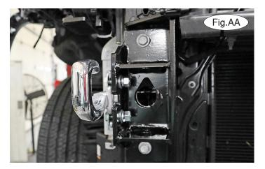
20. Place two 7/16" flat washers and Loctite over two 7/16" x  $2\frac{1}{2}$ " bolts. Loosely install the bolts into the tow hook mounts and finish each bolt with a small 7/16" flat washer, 7/16" lock washer and 7/16" nut (Fig.AA). With the assistance of a second person, apply forward pressure to the tow hook on each side (Fig.BB) and tighten the hardware to the specifications.
