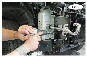
16. On each side, using a  $1\frac{1}{2}$ " hole saw and the front cutout on the baseplate as a guide, cut a frame access hole (Fig.W).
