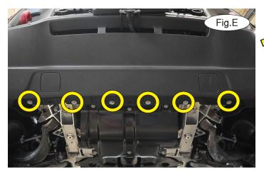
3. For Trailhawk Models only: Remove six 10mm bolts attaching the fascia to the frame (Fig.E). For all other **models**: On each side, remove four 10mm bolts and one 8mm screw attaching the splash shield to the frame (Fig.F – circles). *Note:* There is one extra 10mm bolt on the driver's side (Fig.F – arrow). Let the splash shield hang down for now. *Note: Due to manufacturing variances, there may be an additional 13mm bolt that needs to be removed (Fig.F — inset), or two plastic fasteners.*
