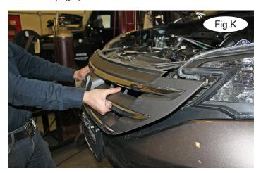
7. With a firm grip on the grille, pull hard and straight out on it to release it from the two yellow clips near the headlights and the four yellow clips along the bottom of the grille (Fig.K). On each side, pull out on corner of the fascia to remove it from the locking strip as indicated by the yellow lines in Figure L) and then a screwdriver to release the yellow clip shown in Figure M.
