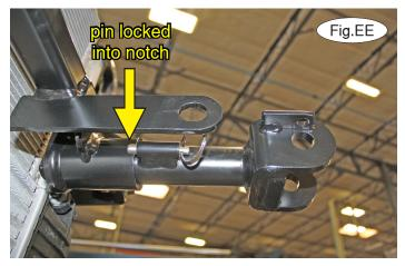
22. On each side, insert the removable front bracket arm into the front receiver 90 degrees from its final towing position, depressing the spring-loaded pin against the receiver (Fig.DD). Now, twist back 90 degrees until the spring-loaded pin snaps into place in the notch on the receiver, locking the arm into place in its final towing position (Fig.EE).
