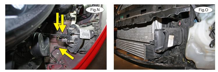
10. Pull forward on the fascia to gain access to the fog lights and disconnect them (Fig.N). Also, locate the ambient temperature sensor (on the passenger side only) and disconnect it and its wiring loom. *Note:* do not start the vehicle when the temperature sensor is unplugged because it could cause the 'Check Engine' light to illuminate.
