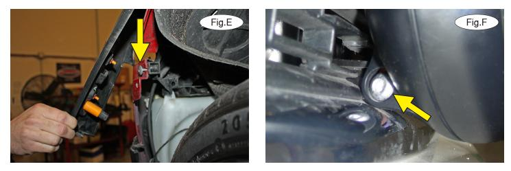
3. On each side, release the front clips (depending on year and model, the number will vary) along the front edge of the fender flare to gain access to the T25 Torx bolt (Fig.E) and then remove it.
