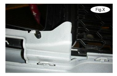
20. Hold the fascia in place over the main receiver brace and trim the fascia using Figure W as a guide for trimming.
