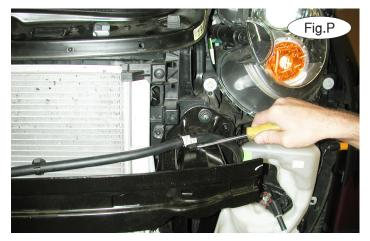
12. On each side of the radiator, remove one plastic fastener attaching the water line to the top of the bumper core (Fig.P). *Note:* due to manufacturing variances, not every vehicle will be equipped with this water line.
