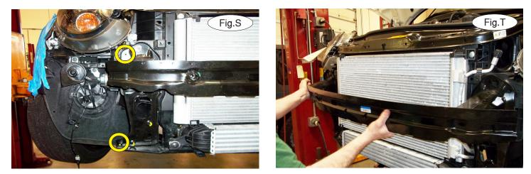
15. On each side, remove two T20 Torx bolts attaching the bumper core to the core support (Fig.S).
