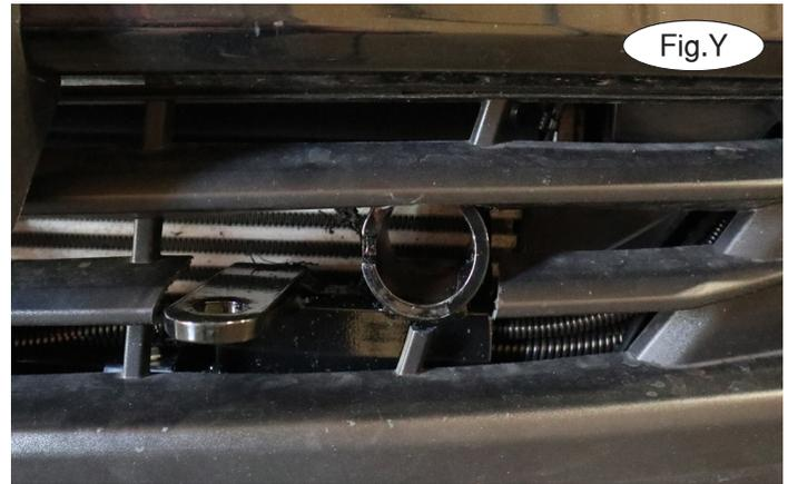
18. For '18-'21 models: Trim the fascia on each side as shown in Figure X (driver's side). For '22 models and later: Trim as shown in Figure Y (driver's side). *Note: If your vehicle is equipped with an additional plastic air dam, you will need to either remove the entire piece as shown (Fig.Z – arrow) or trim it to allow clearance for the main receiver brace.*
