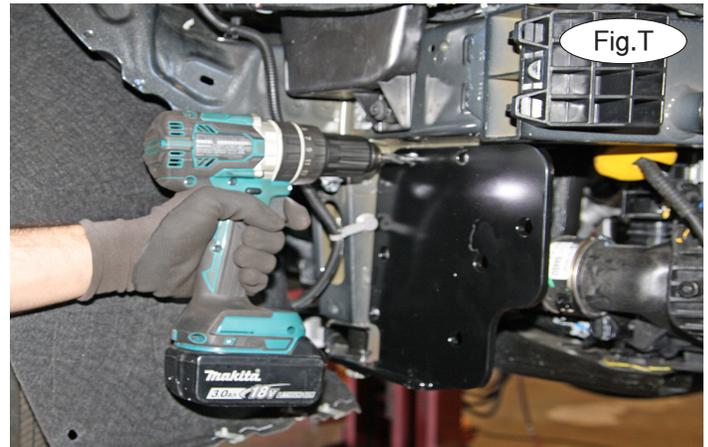
12. Repeat steps 10 and 11 for the driver's side, and then torque all of the installed bolts on both sides.
