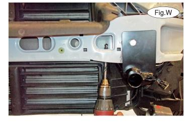
ceiver brace as a template, drill up through the bumper core (Fig.W). Bolt up through the main receiver brace and bumper core using a  $\frac{1}{2}$ " x 134" bolt and finish with a 3/16" x 11/2" x 3" backing plate,  $\frac{1}{2}$ " lock washer and nut.
