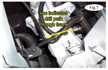
15. On each side, locate the pre-existing hole on the outside of the frame rail, as well as the corresponding hole on the inside of the frame rail. Using a ½" x 12" drill bit, enlarge the two holes in the frame rail (Fig.S and Fig.T). Make certain you use a sharp drill bit. *Note:* use a piece of metal as a buffer between the drill bit and the engine components.
