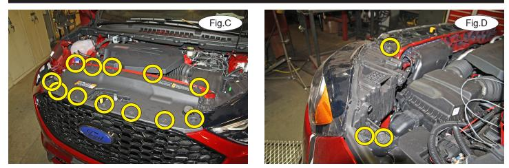
1. Important: please use all supplied bolts and parts and read all instructions carefully before beginning this installation. The majority of questions you may have can be answered within the text, and proper installation will ensure safe and secure travel. Now, begin the installation. Remove 12 plastic fasteners attaching the radiator cover to the fascia (Fig.C). Remove the cover and set it aside for now.
