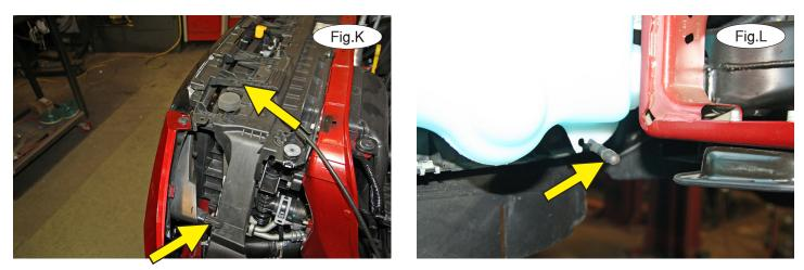
8 On each side, release two plastic clips attaching the fascia to the radiator core (Fig.K). Disconnect all wiring harnesses and the washer hose for the front camera. *Note:* You will need to secure the hose in some way so that it doesnt leak. We suggest placing a rubber cap over it, as shown in Figure L. Set the fascia aside for now.
