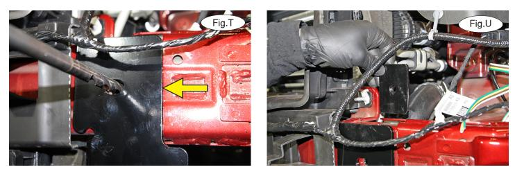
15. Ensure that the upper mount of the baseplate is flush with the raised end of the bumper core as shown (Fig.T – arrow). Now, use a  $\frac{1}{2}$ " drill and the upper mount of the baseplate as a template to drill through the face of the bumper core (Fig.T). Make certain you use care to avoid drilling into critical engine components.
