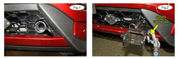
20. Now, on each side, push the upper mount toward the upper corner and torque the  $3\frac{1}{2}$ " bolts. Then, torque the  $4\frac{3}{4}$ " bolts,  $4\frac{1}{2}$ " bolts and finally, the 1" bolts.
